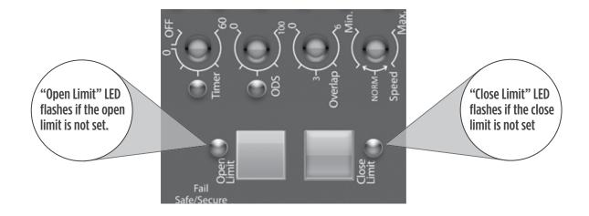
**Tip:** The gate can be moved electronically with the "Open", "Stop" and "Close" buttons on the Control Board or manually by following the instructions on page 11.
