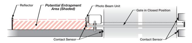
Consult the installation manual for the UL325 device (photo beam or like) for detail information about the usage, installation and maintenance.
