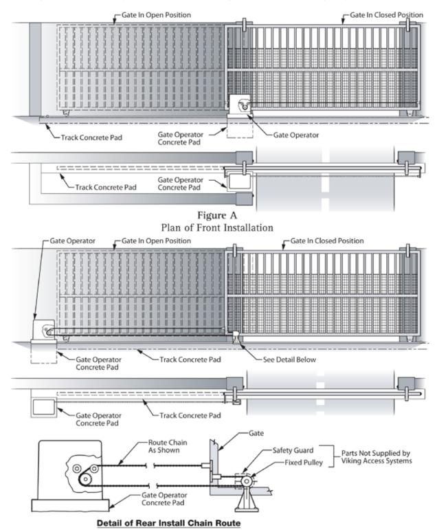
Figure B Plan of Rear Installation
